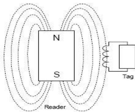
Figure 5: RFID Near Field Methodology
