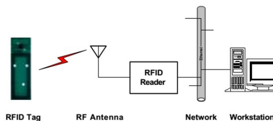
Figure 2: RFID Components
