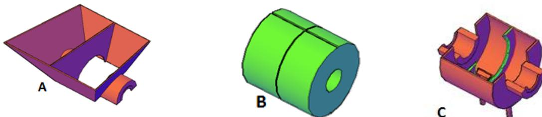
*Figure 2. Component of the planter, A seed and fertilizer hopper, B seed and fertilizer metering dives and C seed and fertilizer metering dives housing.*
