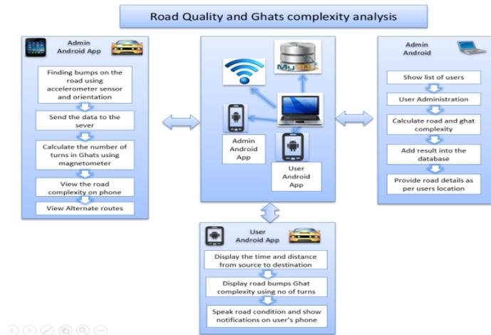
Figure 1: System Architecture Design
