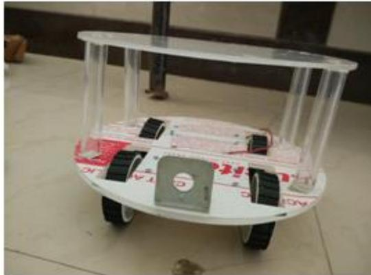
*Fig. 6(a) Chassis design of Master using layered approach*
