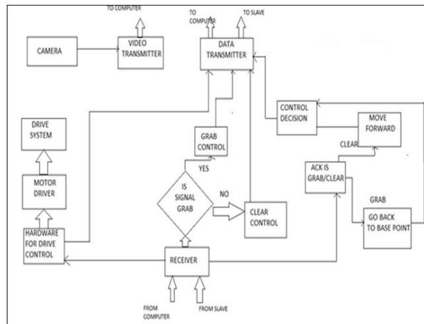
**Fig. 8 Working diagram of Master**
