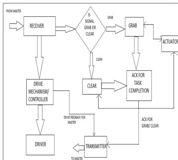
**Fig. 9 Working mechanism of Slave**
