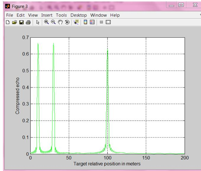
Fig. 3 Recovery signal from received signal by matched filter (echo)
