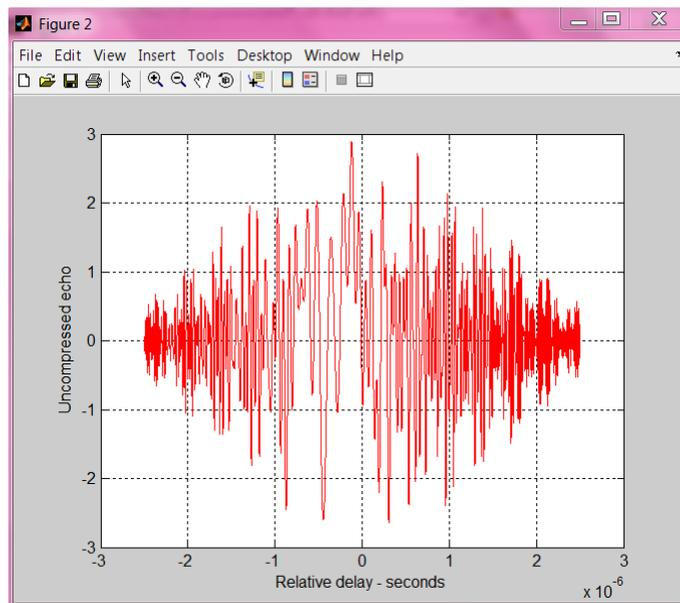
**Fig. 2 Uncompressed Received signal (echo + noise)**
