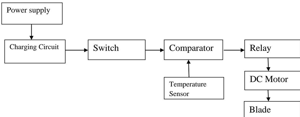
Figure 1 Block Diagram of Existing System
