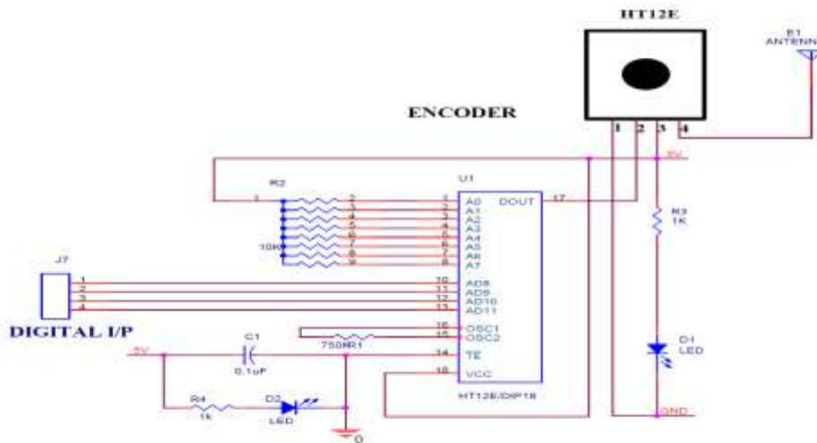
Figure 4 Transmitter with Encoder
