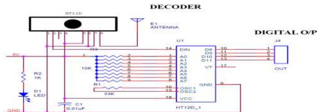
Figure 3 Receiver with decoder
