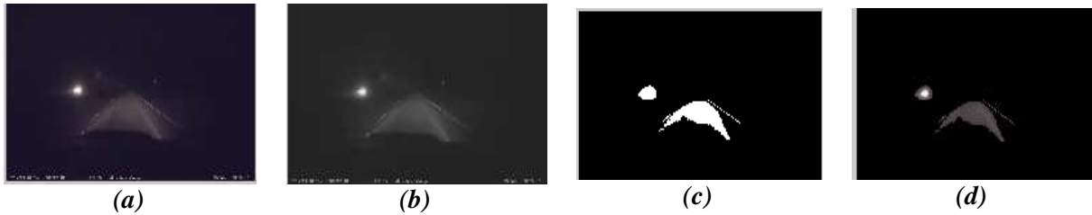
Figure 4: (a) Input Frame 334 and 574; (b) Luminance Image; (c) Binary Image; (d) Segmented Object in Current Frame in Video 2.
