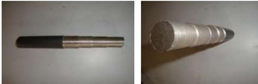
*Fig 6. Mild Steel (Work piece) after machining on Lathe*
