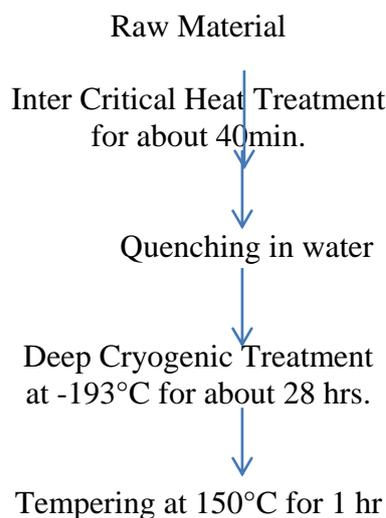
*Fig 5 Process Flow Chart of Deep Cryogenic Treatment*
