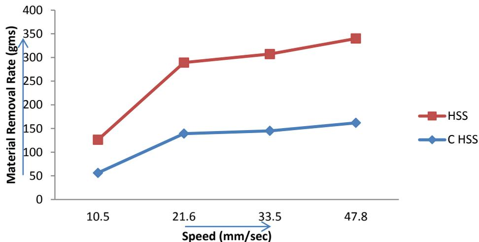
Figure No 11 MRR attained using cryogenic treated and non treated HSS Tool.
