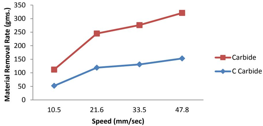
Figure No 10 MRR attained using cryogenic treated and non treated Carbide Tool
