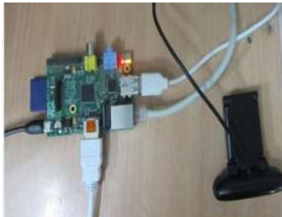
Fig 4: Connection Of USB Camera With Raspberry Pi
