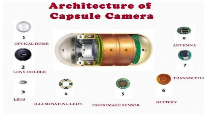
Figure 2. Architecture of capsule endoscopy[4]
