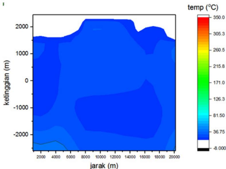
Figure 5. Steady state model shows subsurface temperature distribution slice8 in the 100,000<sup>th</sup> year
