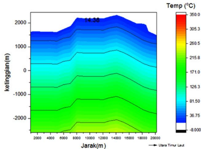
Figure 4. Modeling steady state distribution of subsurface temperature slice 8 in year 0
