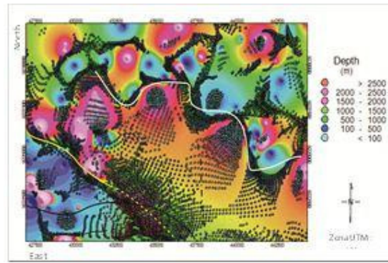
Figure 6 Overlay of Euler de-convolution results with a second vertical gradient map
