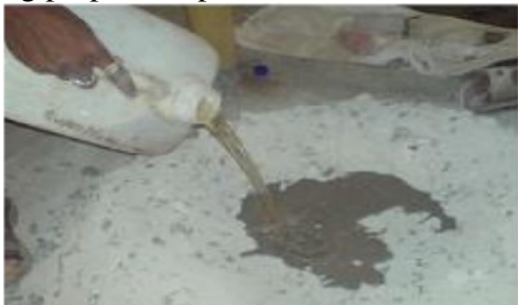
Figure 5.1 Mixing of Geopolymer Concrete.
