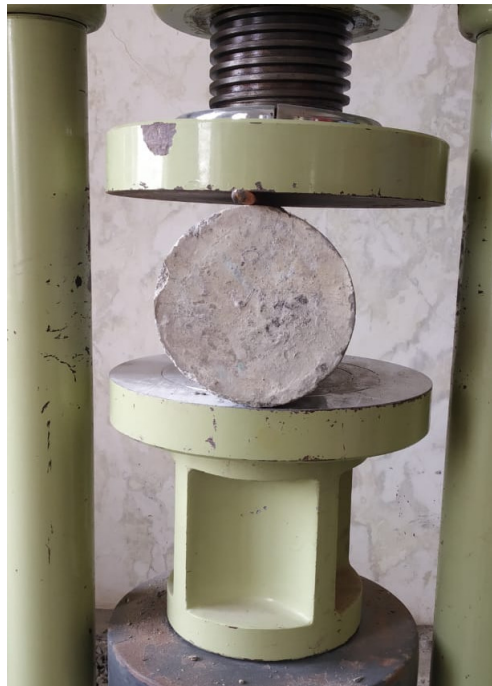
Figure 2. Split Tensile Strength Test
