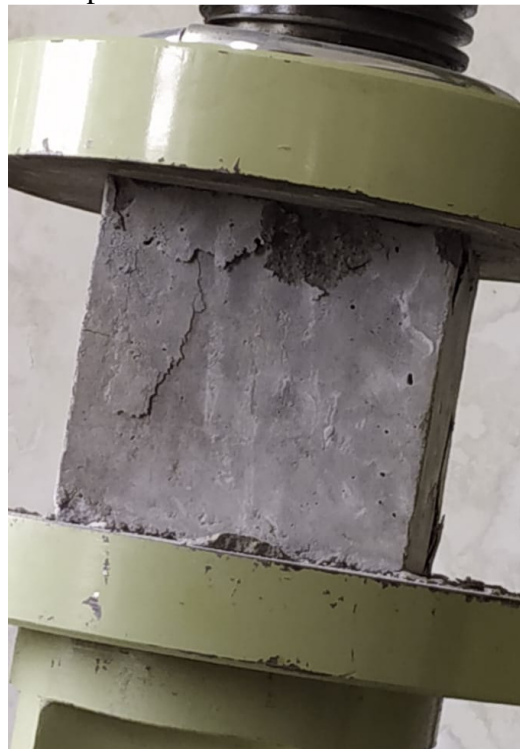
Figure 1. Compressive strength tests
