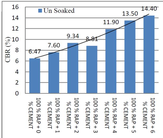
**Fig. No. 1 - Unsoaked CBR value of RAP with varying % of cement**
