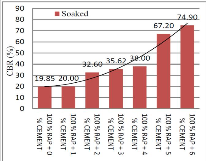
**Fig. No. 2 - Soaked CBR value of RAP with varying % of cement**
