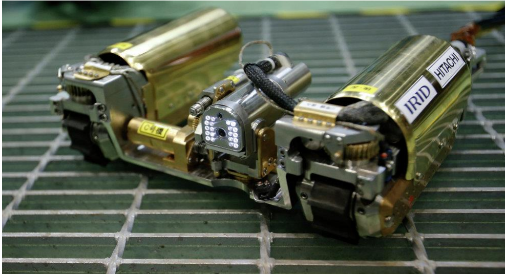
Fig.4: Hitachi Developed a Snake Like Robot for Investigation in the Reactor Core. Courtesy: Associated Press Photo.
