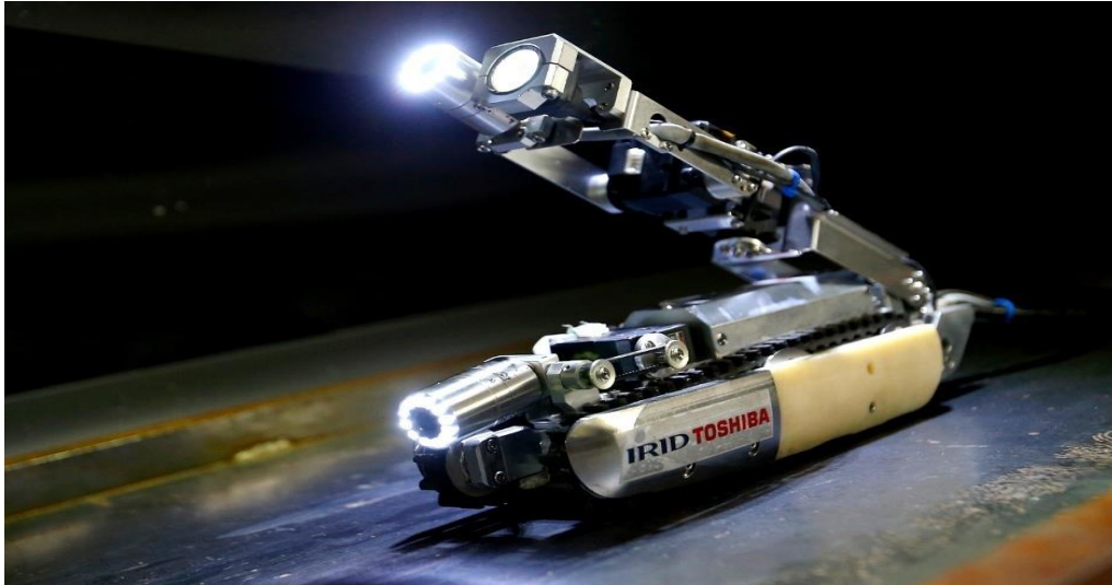
Fig.5: Toshiba's Revolutionary Scorpion Robot to Explore the Fukushima Reactor. Courtesy: Technocrazed.com
