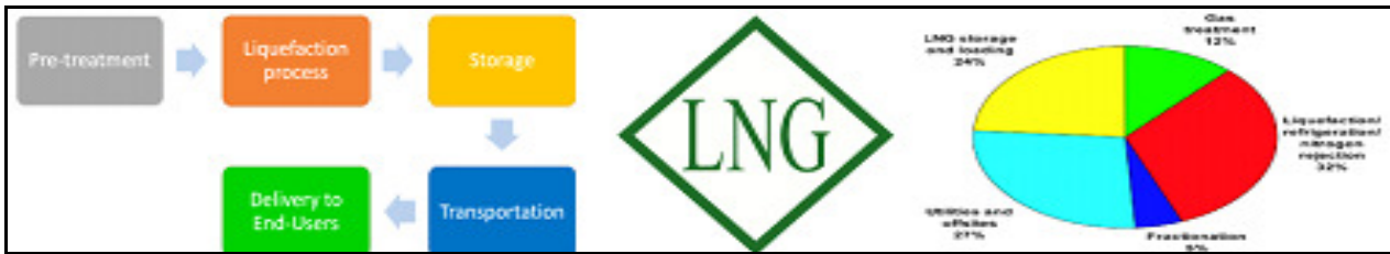
Figure (3):- LNG's liquefaction / refrigeration and nitrogen rejection is 32%, Utilities & offsets 27%, Storage & loading is 24%, gas treatment 12%, and fractionation 5% [4].
