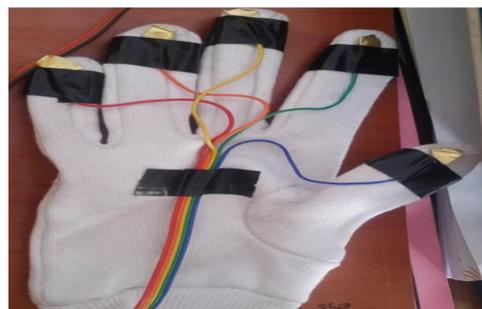
**Fig.5** Touch sensor with glove
