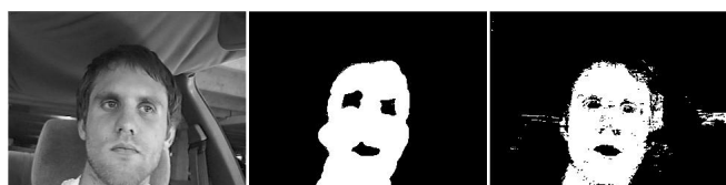
Fig. Skin color predicate training. The first image is the input image, the second shows the manually selected skin regions, and the third shows automatically detected skin regions.
