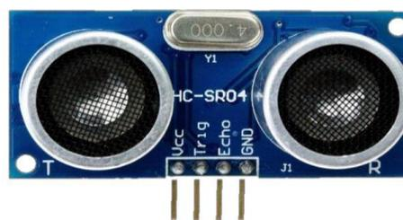
Fig 2 - Ultrasonic sensor HC-SR04
