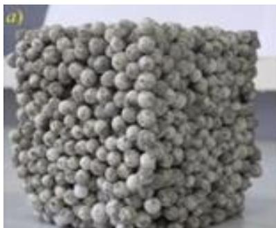
**Fig.1 Expanded polystyrene concrete block**
