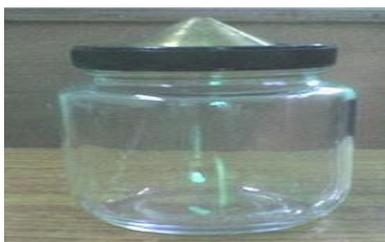
Fig.2 Pycnometer Apparatus
