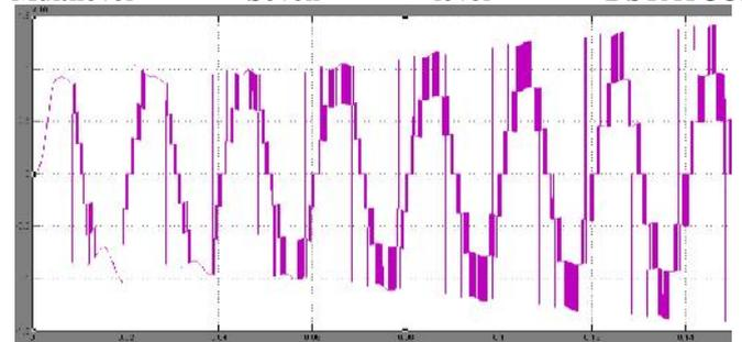
Fig 15 Seven level output Voltage
