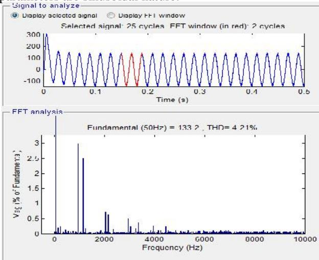
Fig.12 FFT Analysis of Source Current A -Phase with Grid Connected system with DSTATCOM
