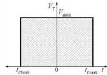
Fig 7: The V-I characteristic of D-STATCOM
