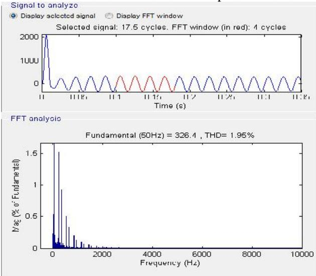
Fig.17 FFT Analysis of source current with compensator using MLI based DSTATCOM
