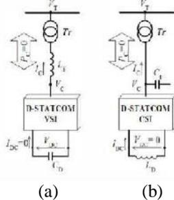
Fig 3: General topology of VSI-based and CSI-based DSTATCOM
