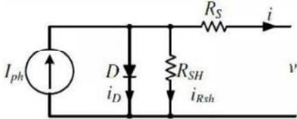
Fig 8: Electrical characteristics of PV Cell model.
