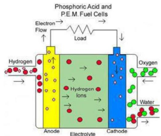
Fig.9. Basic schematic of fuel cell operation
