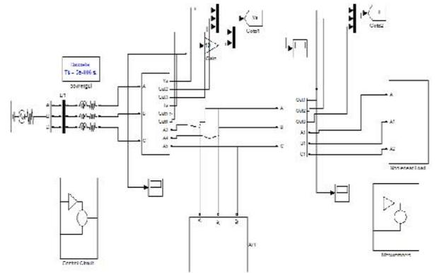
Fig. 13 Matlab/Simulink Model of proposed Grid Connected Pv System with Multilevel DSTATCOM
