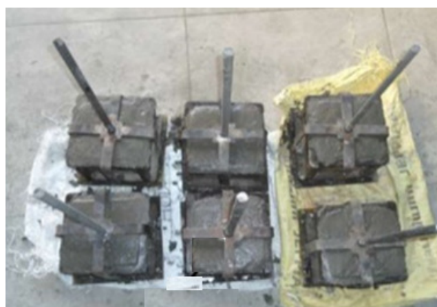
Fig.2. Casting of cube.
