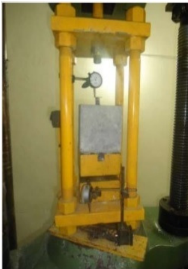
Fig.4. Arrangement of pull-out specimen in UTM
