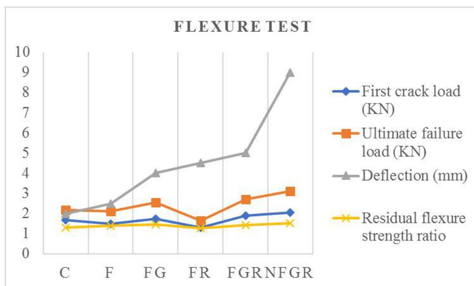
Figure 8. Flexure strength results
