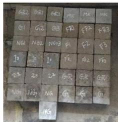
Figure 4. Mortar cubes
