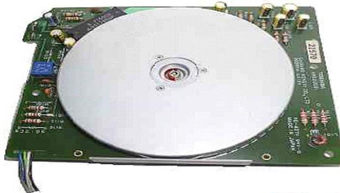
Fig. 1.3 Brush less DC (BLDC) MOTOR Drive
