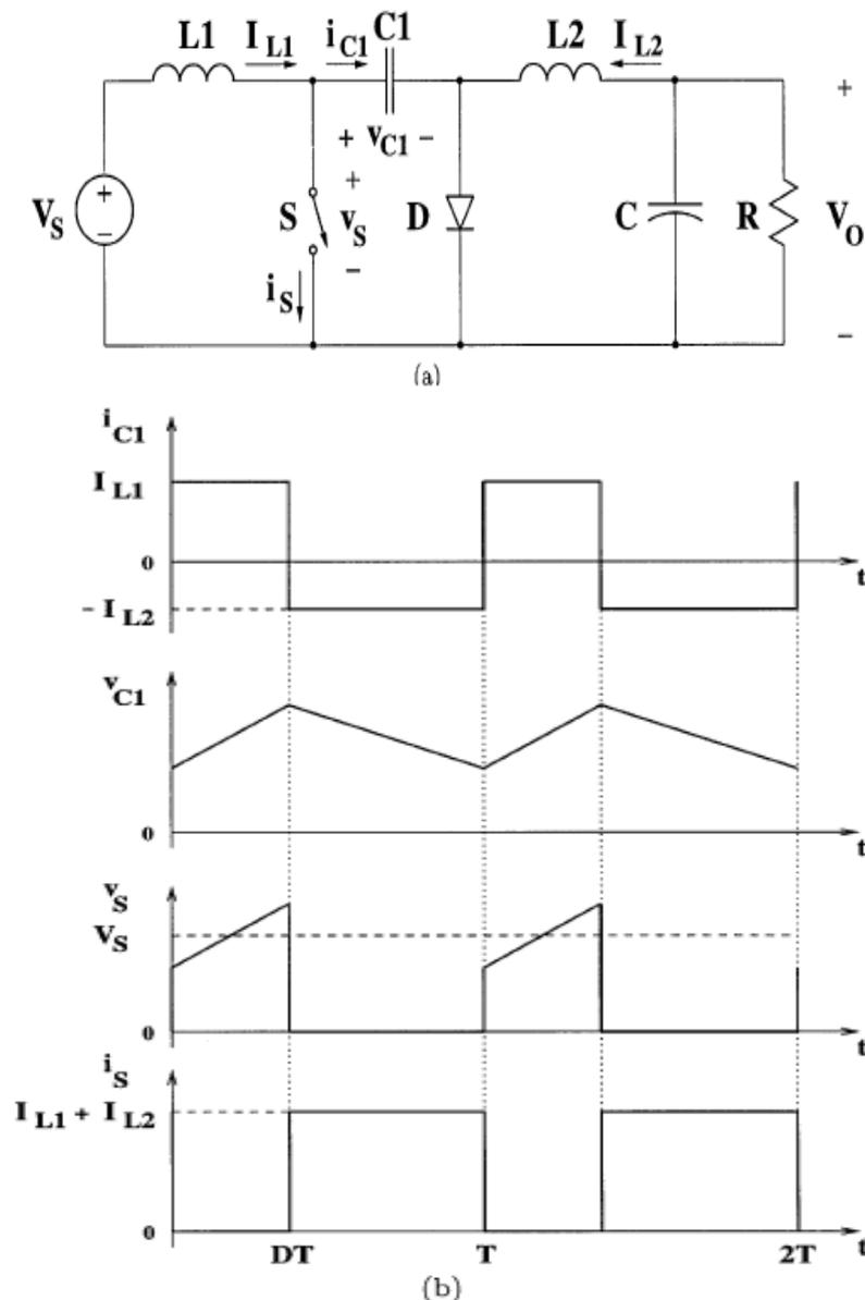
**Fig. 1.1 CUK CONVERTER : (a) CIRCUIT DIAGRAM; (b) WAVEFORMS.**
