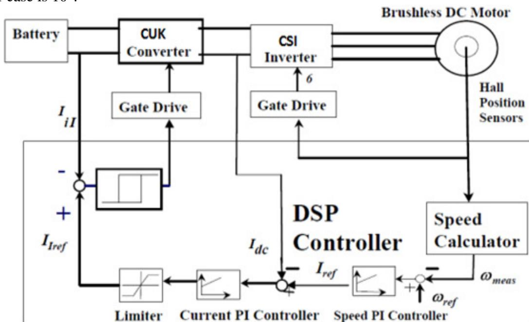
Fig. 1.2 BDLC MOTOR USING CUK CONVERTER & CSI INVERTER
