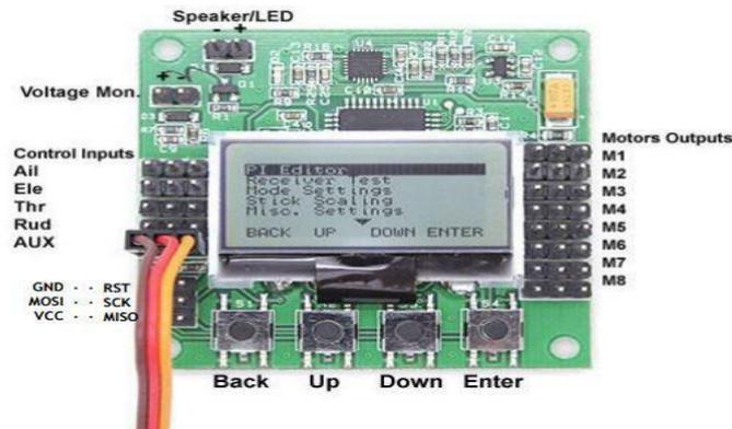
Figure 3: KK Multi rotors Control Board
