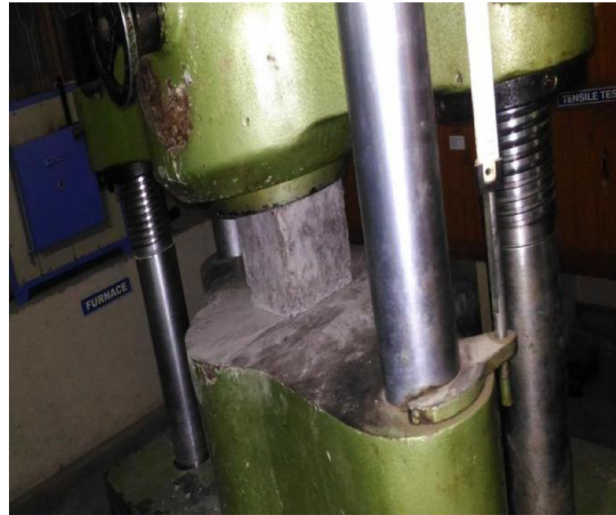
Figure2. Testing of cube
