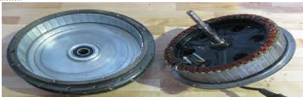
Figure 2: Image for the hub motor internal arrangement
