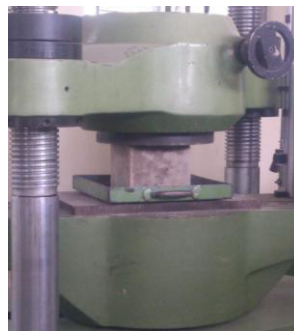
Fig 4.1 compressive strength test
