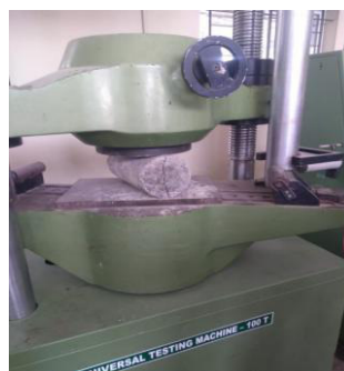
Fig 4.2 split tensile strength test
