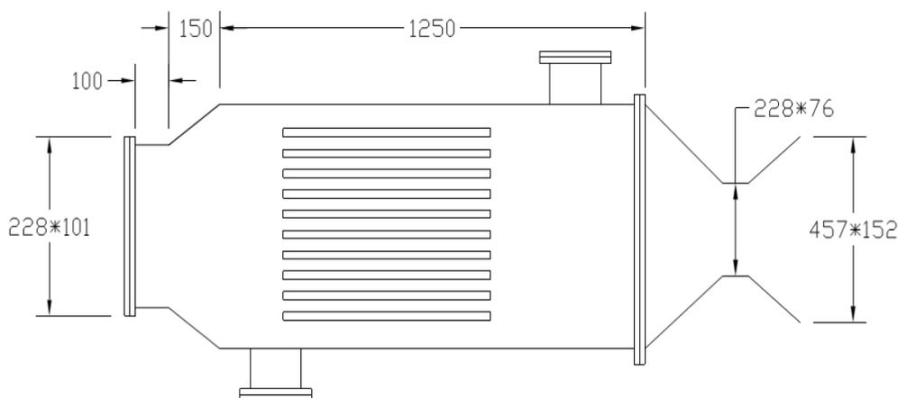
**Fig 2.** Dimension of the Modular Heat Exchanger
