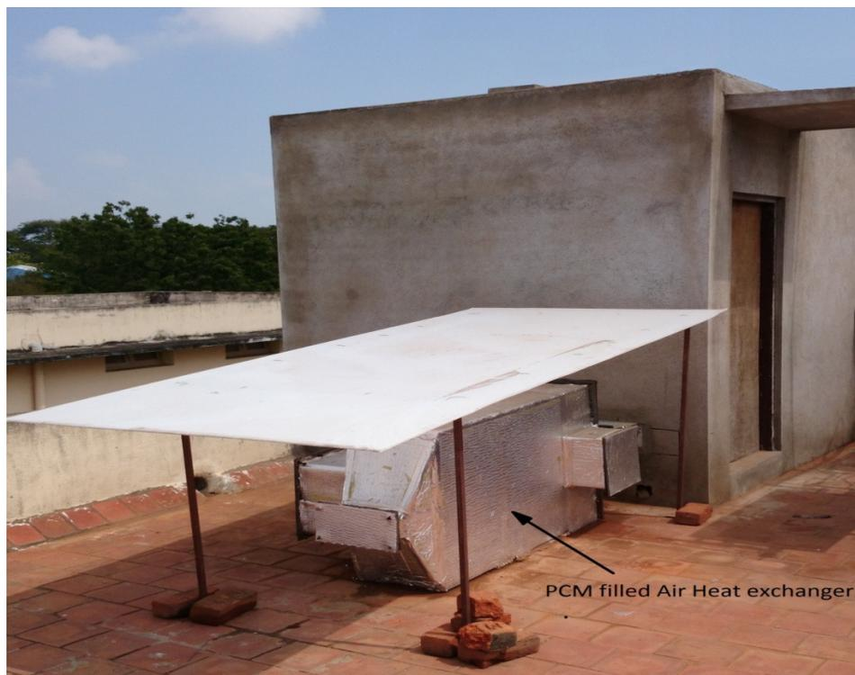
**Fig 1:** A photographic view of the experimental cabin with the modular heat exchanger
