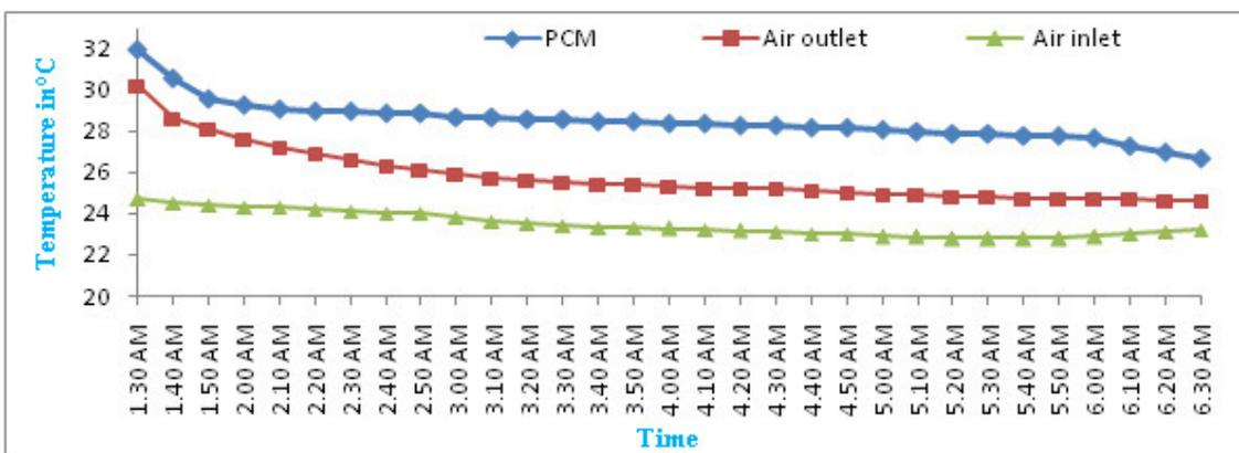
Figure 3. Temperature distribution during charging
