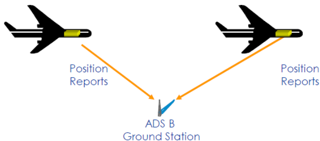
Figure 1 Automatic Dependant Surveillance
