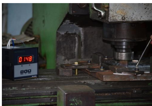
Fig. 2 Friction stir welding experimental setup with provision to measure temperatures using thermocouples
