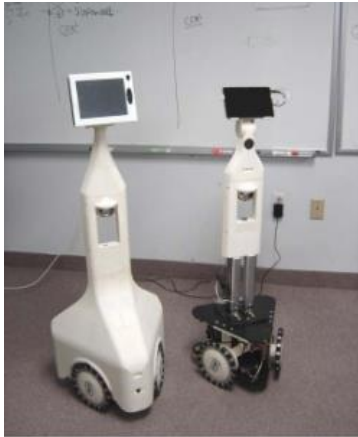
Figure 1. The Robotic Nurse modular prototypes. A robot without the cover demonstrates a movable platform system.
