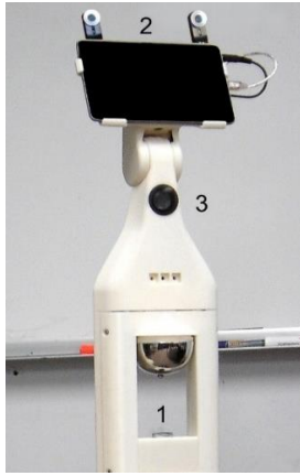
Figure 4. Robotic Nurse top devices: 1—360°-panoramic viewing; 2—stereo pair; 3—speaker.
