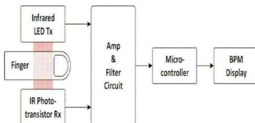
Fig 3. Functional block diagram of the heart rate sensor
