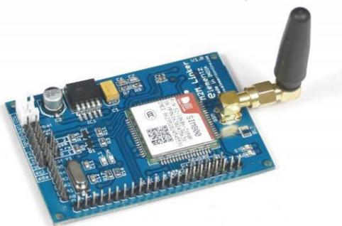
Fig 3: GSM MODULE
