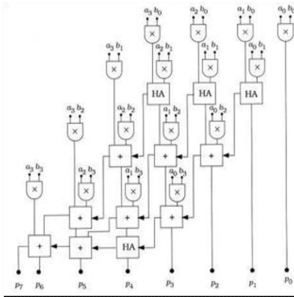
The delay associated with the array multiplier is the time taken by the signals to propagate through the AND gates and adders that form the multiplication array. Delay of an array multiplier depends only upon the depth of the array not on the partial product width.
